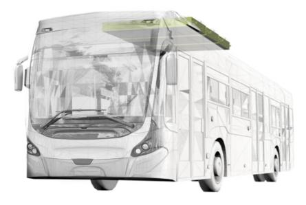
AKASOL's high-performance battery systems allow versatile positioning depending on the model of bus. (Graphic: AKASOL)
